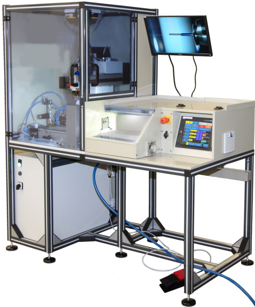
Varnishing unit with three-axes guide and pressure based varnish dosing system
