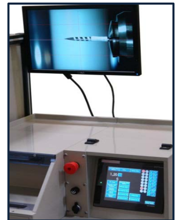
Monitor to check varnishing
